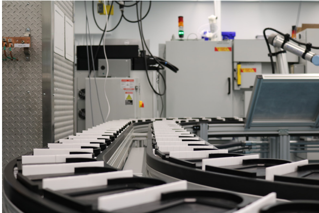
A Conveyance system: A U-shaped conveyance system carries material specimens from station to station. The inner and outer tracks move in opposite directions, allowing samples to move clockwise or counterclockwise throughout the system as needed.
