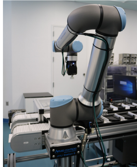
B UR10e robots: Each robot has a reach of 51.2 inches and is capable of carrying a 27.55 lb payload. Equipped with vacuum grippers, the robots move material specimens from the conveyance system to their proper positions for processing, testing, and characterization.
