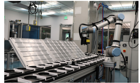
Figure 11: UR10e robots are installed at each station in the AIMD Lab. The robots are fitted with vacuum grippers to facilitate specimen handling.
