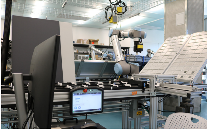
C Station manning infeed/outfeed: Samples (each mounted within a rectangular sample frame) begin and end their journey on these large trays, where a robotic arm adds them to or removes them from the conveyance system.
