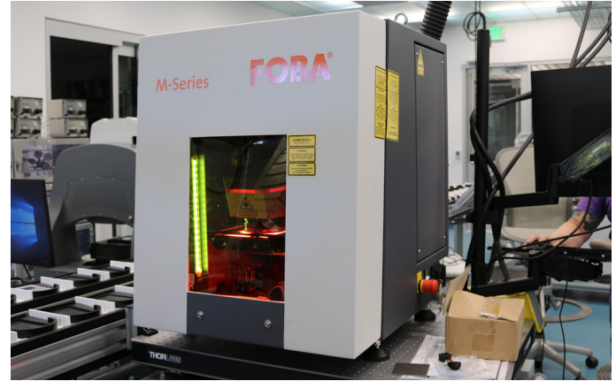
D Laser engraver: A nanosecond pulse laser engraves sample frames with QR codes, allowing samples to be tracked easily throughout the system. This computer-controlled laser has an average output of 20W and is powerful enough to engrave metals, ceramics, and plastics.
