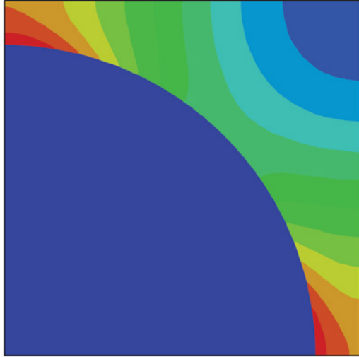
Figure 18: Stress contours corresponding to a unit cell model of a single fiber in a matrix, with debonding at the interface.
