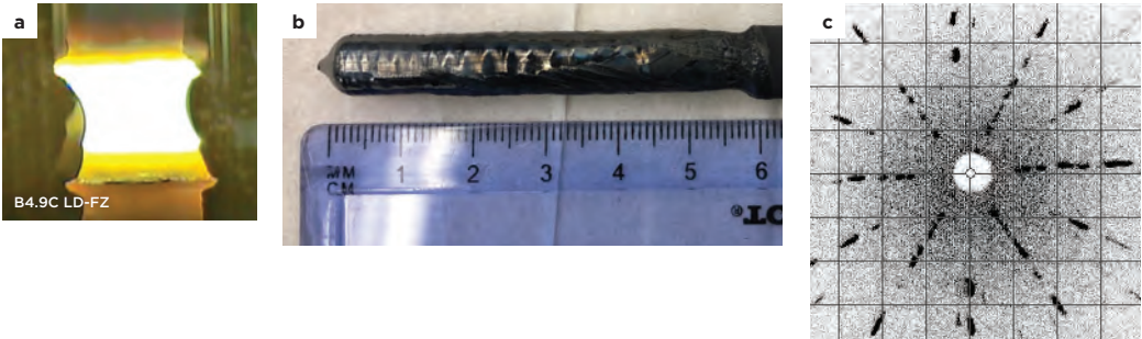
Figure 6: Growth of single crystal Boron Carbide showing (a) an image of the molten zone of the crystal during growth at 2400°C (b) the resulting 8mm crystal boule (c) the measured Laue pattern of the nominal growth direction of the crystal.
