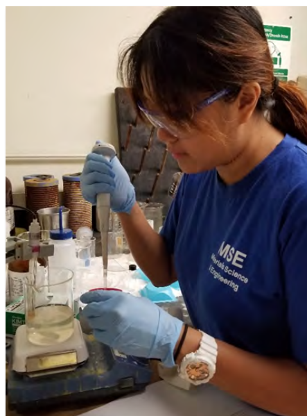
Performing Boron Titration on Boron Carbide Samples
